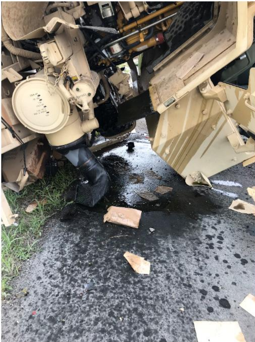
Photo #: 6-Small amount of fuel spilled from LMTV Engine Compartment
