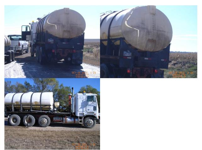
The first two pictures were taken facing south showing the crack in the poly tank where the 10-34-0 leaked out. The third picture was taken facing east, showing the whole truck that was hauling the poly tank in back.
